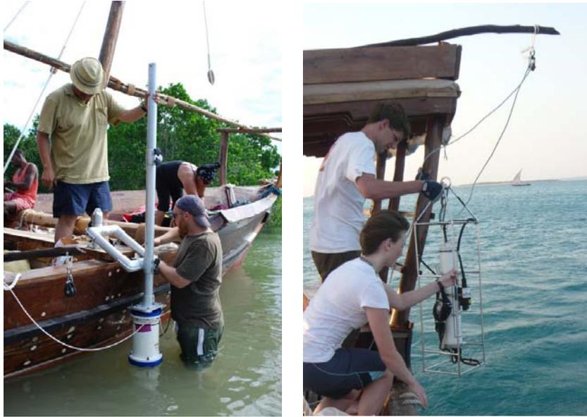
**Figure 3.1** Left panel: Setting the Workhorse Sentinel ADCP and its mount on the research boat. Right panel: Retrieving the SBE-19 CTD from the water after a cast during a transect.
