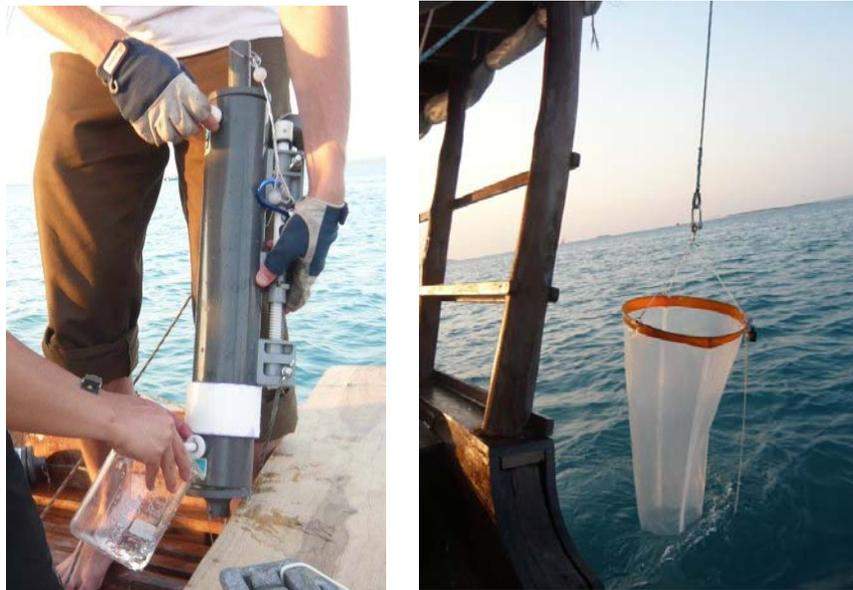
**Figure 3.2.** Left panel: Obtaining subsurface water from a Niskin bottle at a station. Right panel: Retrieving the zooplankton net after a cast during a transect.
